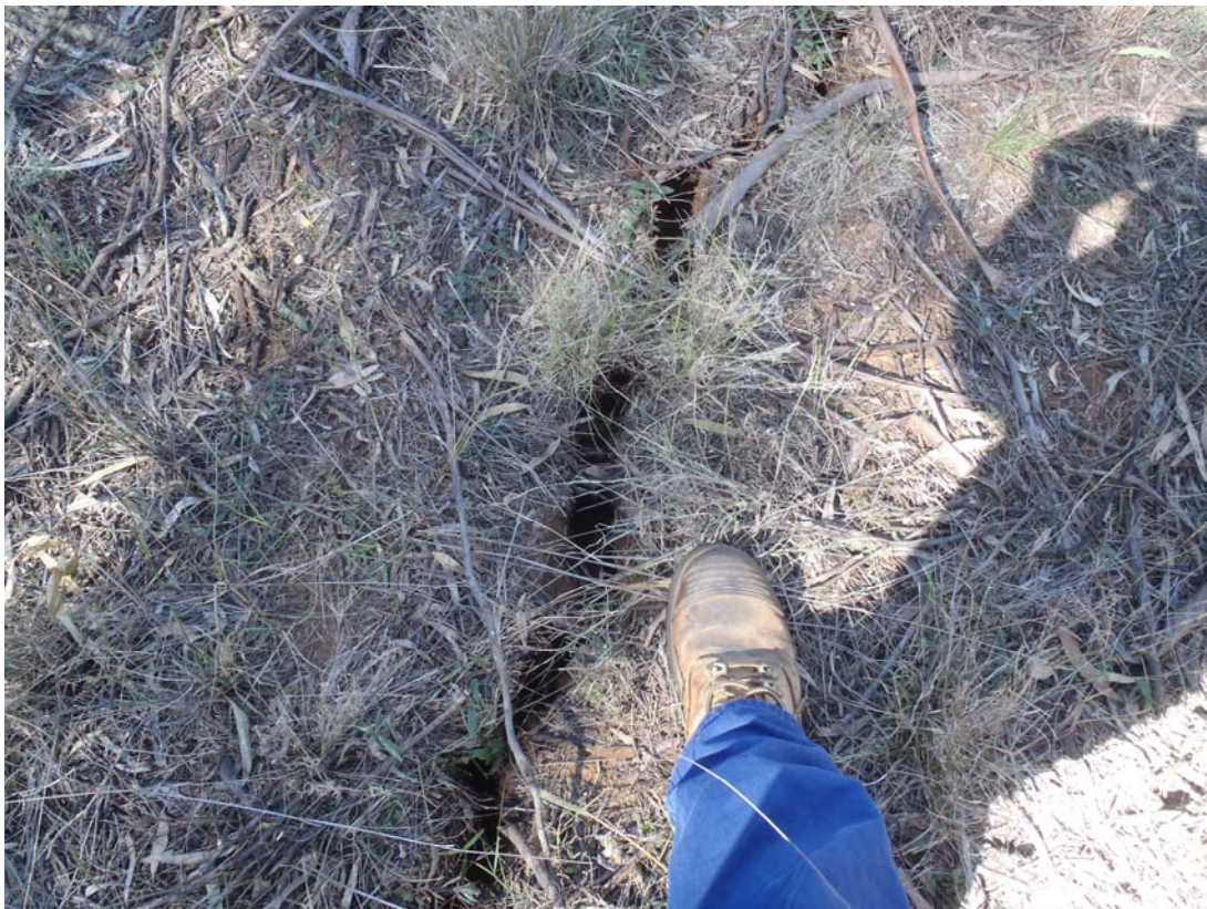
Photo 2: Surface Crack in LW103
